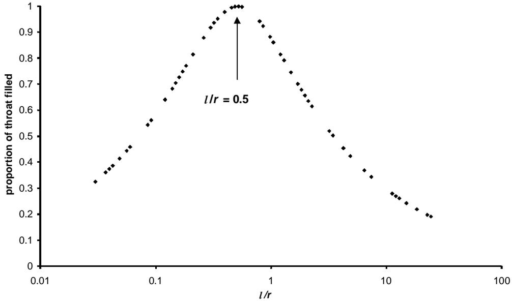
**Figure 10.** For top layer of throats (single capillaries), the proportion of each throat filled after 0.0009  $\mu\text{s}$  shows an optimum  $(l/r)_{\text{opt}}$  ratio of 0.5.
