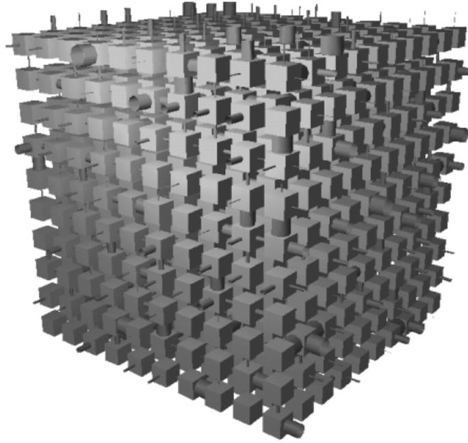
**Figure 11.** Network model unit cell with throat length,  $l$ , of  $1.51 \mu\text{m}$ .
