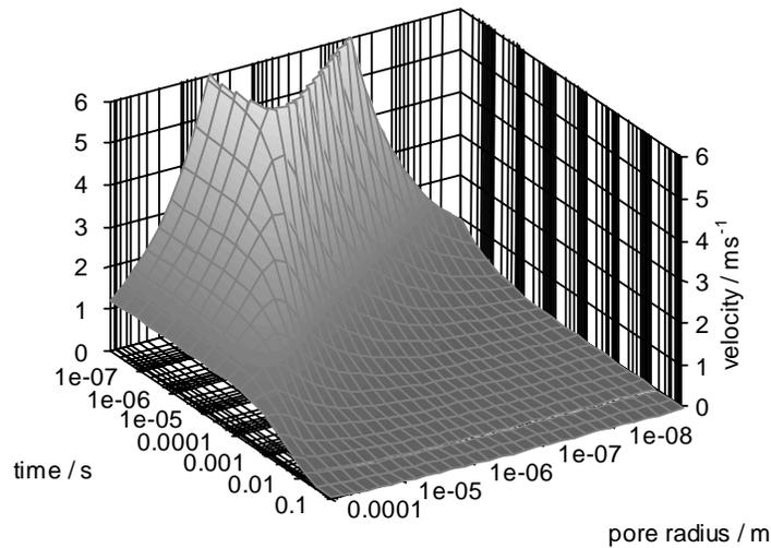
**Figure 3.** Solution to the equation of Bosanquet as a function of time for a range of capillary radii, expressed as imbibition velocity.
