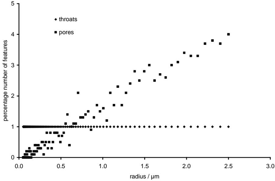
**Figure 12.** Pore and throat size distribution for structure generated with throat radii of 0.05 - 2.50  $\mu\text{m}$ .
