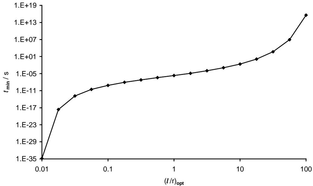
**Figure 8.** The log/log relationship of minimal imbibition time,  $t_{\min}$ , for the equivalent optimal aspect ratio  $(l/r)_{\text{opt}}$  which satisfies eqn [10].
