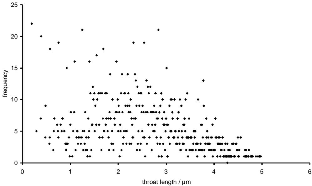
**Figure 13.** Throat length distribution for structure generated with throat radii of 0.05 - 2.50  $\mu\text{m}$ .
