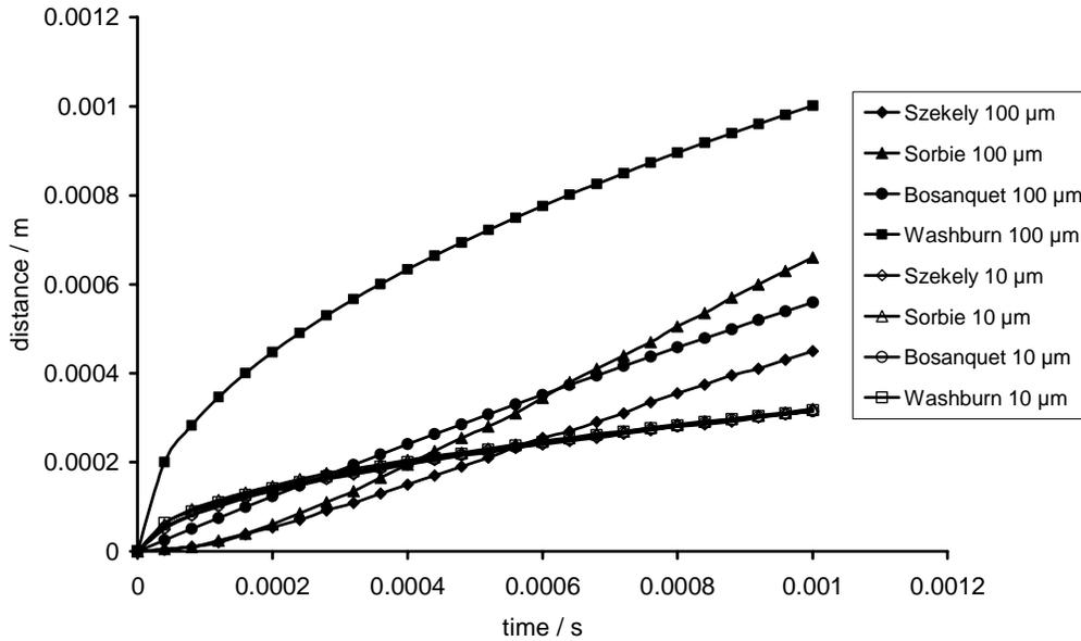
**Figure 2.** Comparisons of solutions to the equations of Szekely, Sorbie, Bosanquet and Washburn for capillaries of 10  $\mu\text{m}$  and 100  $\mu\text{m}$ .
