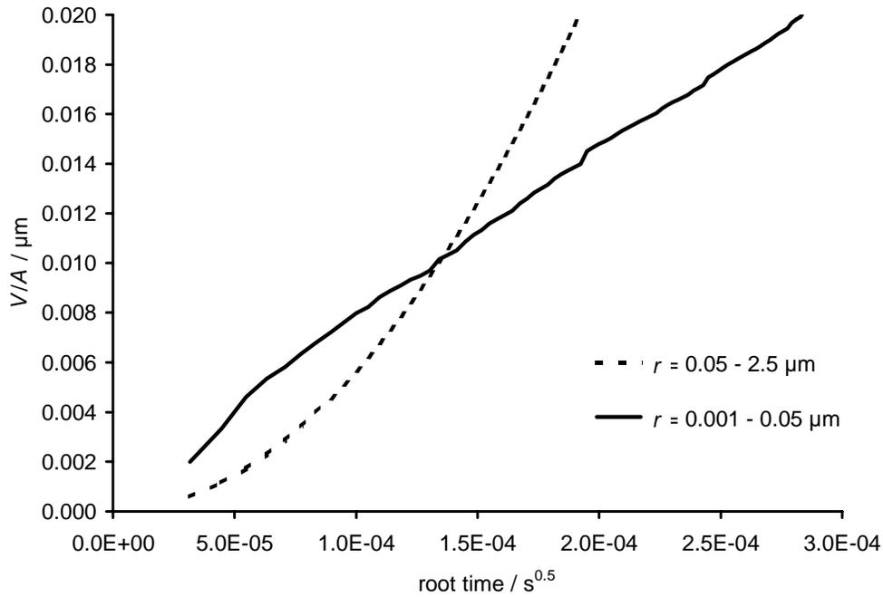
**Figure 14.** Short-time imbibition into a network structure for coarse and fine broad pore and throat size distributions at similar porosity, expressed as volume absorbed per unit area of contact between substrate and fluid supersource.
