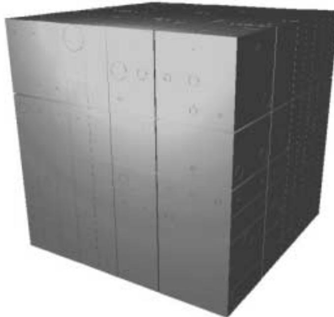
**Figure 9.** Network model unit cell with throat length,  $l$ , of  $0.03 \mu\text{m}$ .
