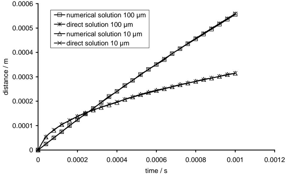
**Figure 1.** Comparison of two solutions to the Bosanquet equation.
