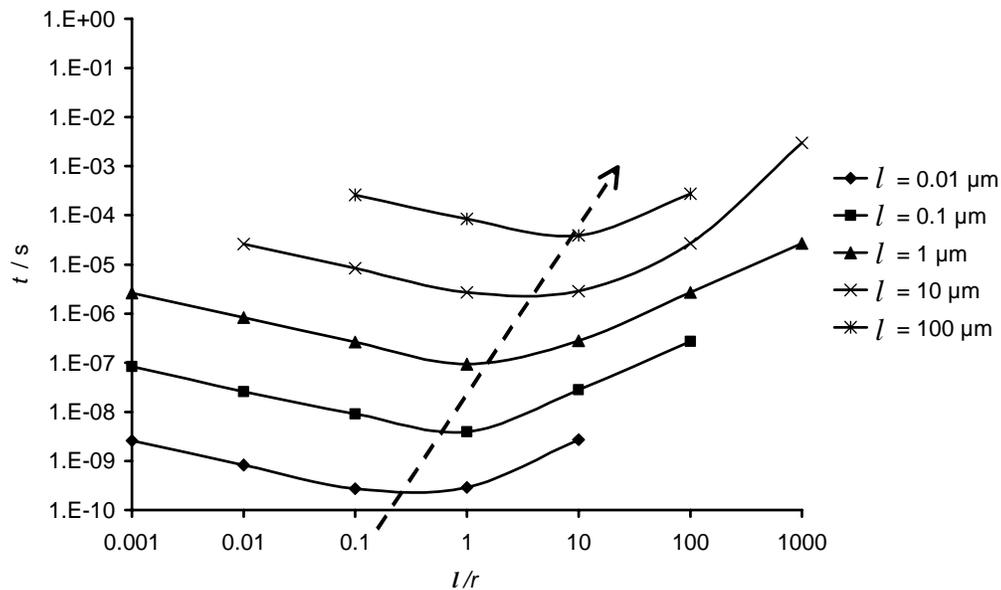
**Figure 5.** Time to fill capillaries for a range of lengths,  $l$ , as a function of aspect ratio,  $l/r$ , using the equation of Bosanquet.
