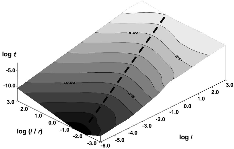
**Figure 6.** Surface graph for time to fill capillaries for a range of lengths,  $l$ , and aspect ratios  $l/r$ .
