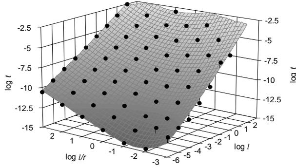
**Figure 7.** Tablecurve 3D surface fit - the data points are calculated values for water imbibition into capillaries.
