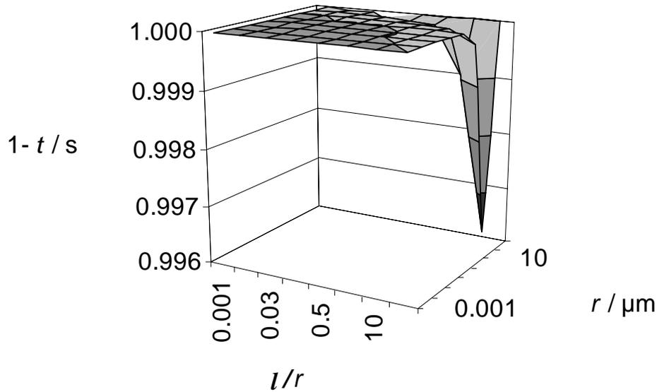
**Figure 4.** Time taken for water to fill capillaries for a range of capillary radii,  $r$ , and lengths,  $l$ , using the equation of Bosanquet.
