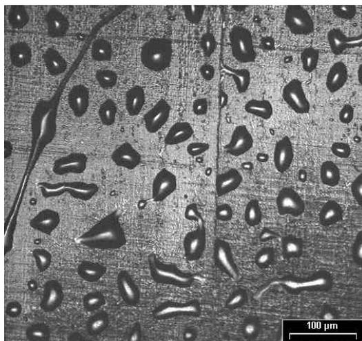
**Fig. 7** Receding ink droplets on PTFE (spinoidal or nucleated dewetting) as seen using confocal laser scanning microscopy in reflected light mode
