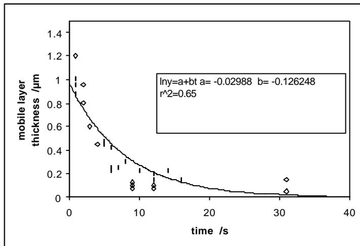
**Fig. 12** Mobile ink layer thickness as a function of time obtained from gravimetric ink splitting experiments
