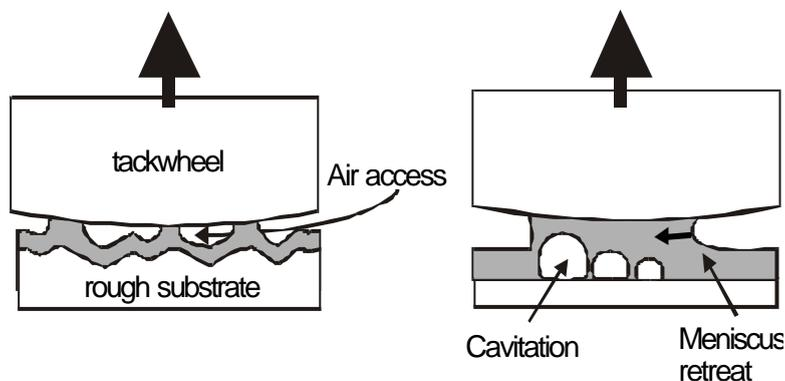
**Fig. 8** Cavitation: on the left, a rough substrate means less ink contact and enables air access, on the right, cavitation at initial fast separation with meniscus retreat as extension progresses, dependent on  $h$
