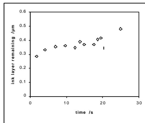
**Fig. 14** Ink layer remaining on paper after tack test as a function of time
