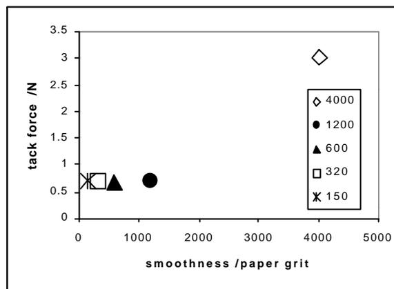
**Fig. 6** Tack force on PTFE in relation to roughness/smoothness. The X-axis shows the sandpaper grit, the value of 4000 is arbitrarily attributed to the untreated smooth surface.
