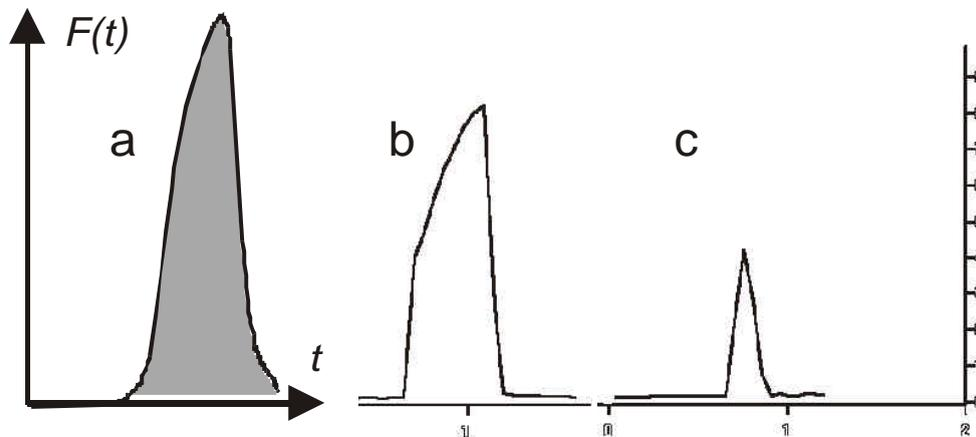
**Fig. 11** a) schematic pull-off curve with integrated area, b) typical curve of Fig. 5 showing 2 regimes: probably cavitation and viscous ones. c) typical pull-off curve as in Fig. 10
