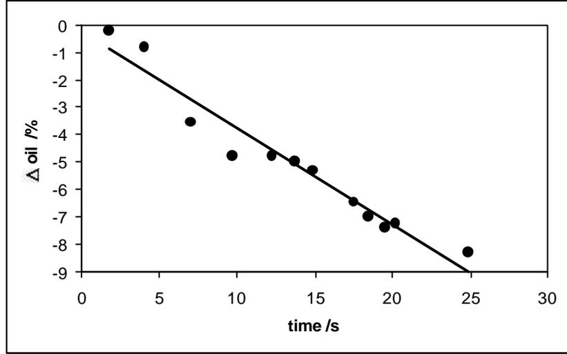
**Fig. 15** The proposed differential oil content of the ink from Eq. 19 as a function of time in contact with the paper surface
