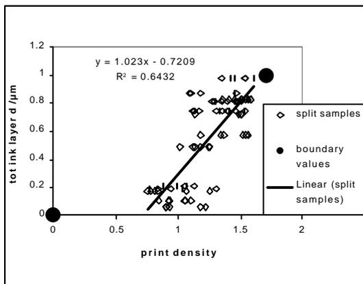
**Fig. 13** Total remaining ink layer thickness as a function of print density
