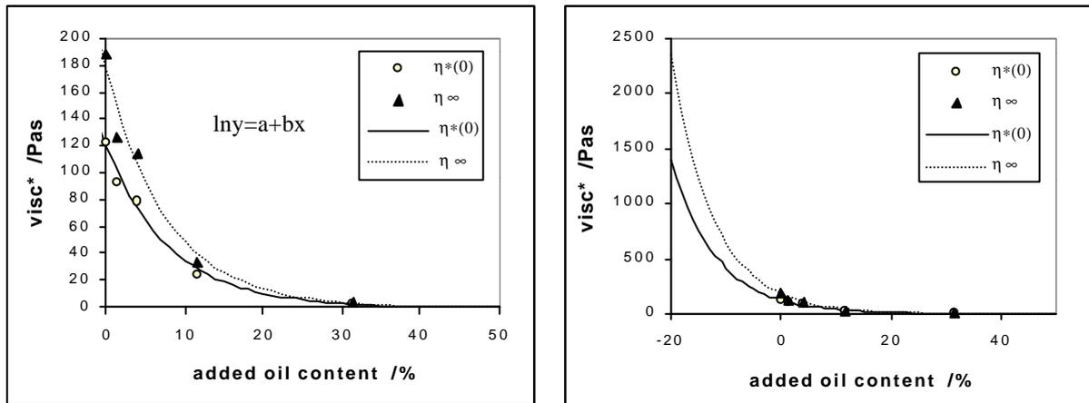
**Fig. 3** Comparison of  $h^*(0)$  and  $h^*(\infty)$  as a function of added oil content of the ink  $\Delta f_{oil}$  (w/w%) - the extrapolation of  $h^*(0)$  ( $a=4.78$ ,  $b=-0.122$ ), on the right, to reduced oil content, is used as the basis for the viscosity comparison with ink tack measurements
