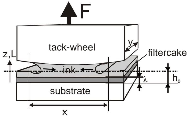
**Fig. 4** Schematic view of tack set-up under the assumed formation of a filtercake with thickness  $I$
