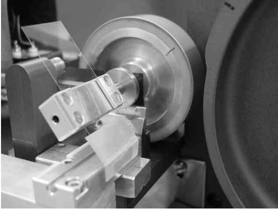
Fig. 4 Detailed view of the mirror (glass slide) and the tack wheel; No.[2] in the previous figure.
