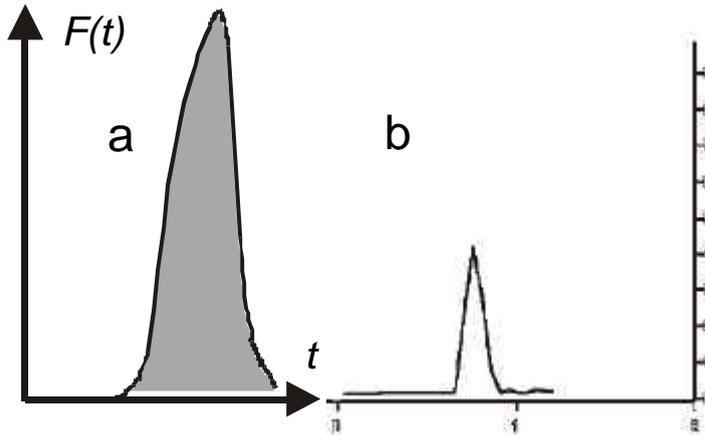
**Fig. 3** a) schematic pull-off curve with integrated area, b) typical pull-off curve asseen in the tack rise region of Fig. 1
