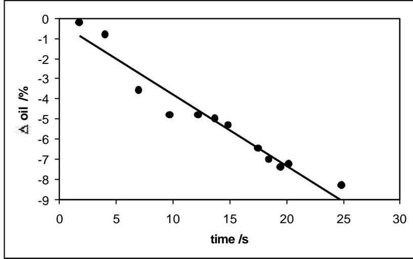
**Fig. 5** The proposed differential oil content of the ink from Eq. 8 as a function of time in contact with the paper surface
