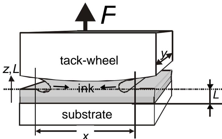
**Fig. 4** Schematic view of tack set-up under the assumed formation of an extensional force.
