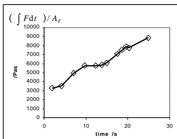
*Fig. 2 The tack rise in the form of a "process viscosity", values are shown in Table 2.*
