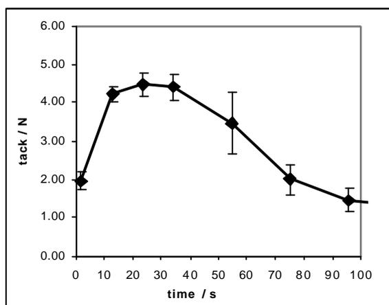
*Fig. 1 Overall mean tack curve for test paper.*
