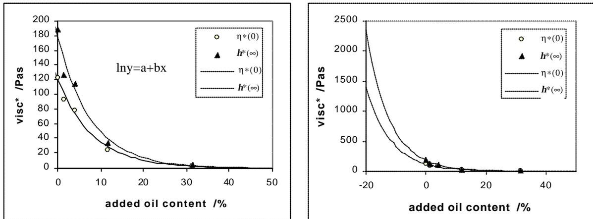
Fig. 3 Comparison of  $h^*(0)$  and  $h^*(\infty)$  as a function of added oil content of the ink  $\Delta f_{oil}$  (w/w%) - the extrapolation of  $h^*(0)$  ( $a=4.78$ ,  $b=-0.122$ ), on the right, to reduced oil content, is used as the basis for the viscosity comparison with ink tack measurement in part II of this paper.
