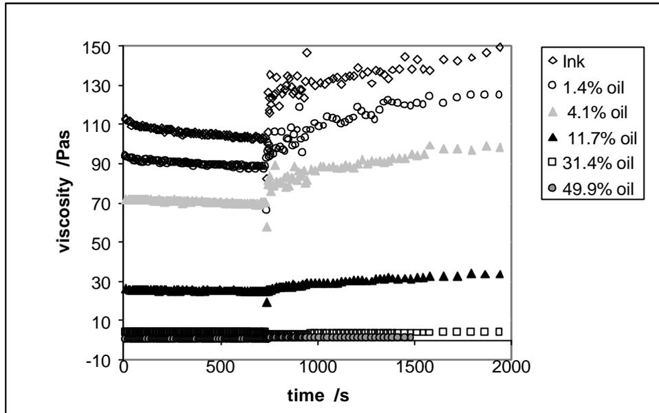
**Fig. 1** Overview of shear viscosity at  $30 \text{ s}^{-1}$  and subsequent relaxation monitored by stress oscillation in the linear visco-elastic (LVE) regime as a complex viscosity,  $\mathbf{h}^*$ .
