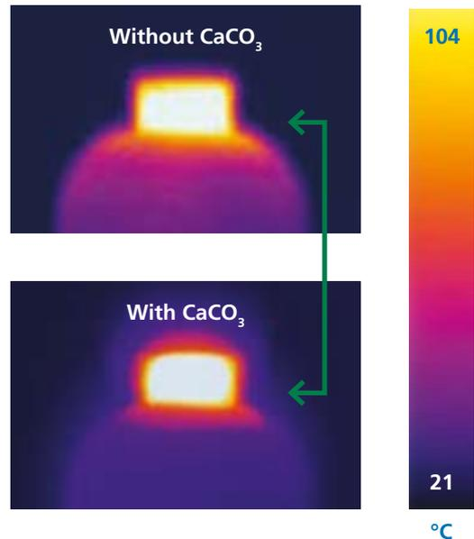
***Omyafilm® has almost 7 x higher thermal conductivity than HDPE***
